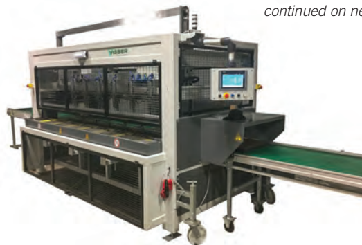
The Visser AutoStix machine removes the challenge of finding and training employees to stick the cuttings at the rooting stations.
