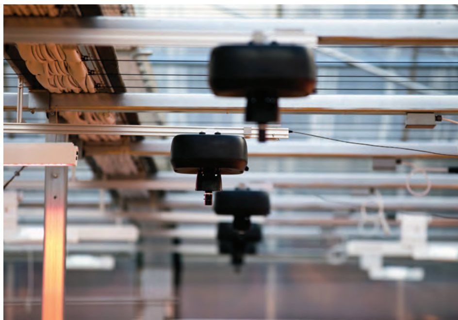
Luna sensors provide data about plant growth, health, water needs, and more. Photo courtesy of iUNU
